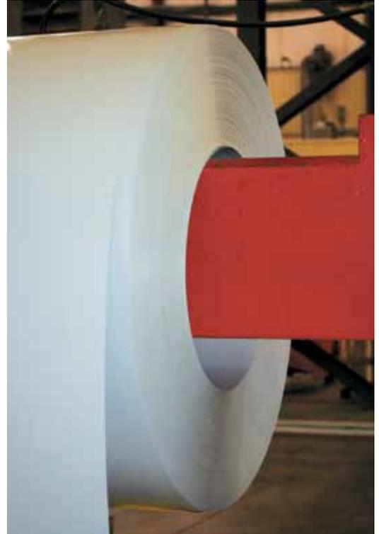
This is how the finished painted coil appears after it has been removed from the paint line's rewind mandrel before packaging. *Photo courtesy of Metal Coaters.*
