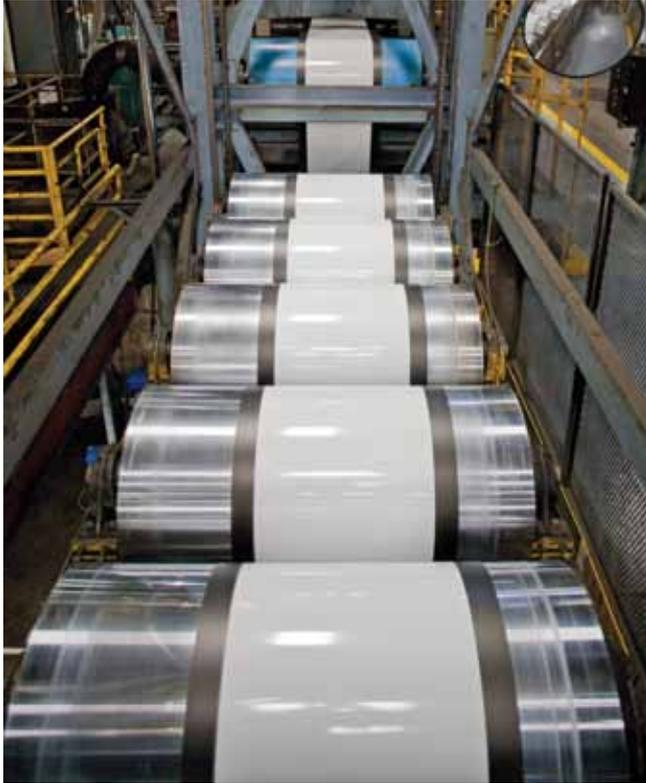
This painted coil with a black base coat and a white "stripe" finish coat is exiting the finish ovens and threading through the exit end accumulator tower. The tower serves as a reservoir of material so when the paint line is temporarily stopped to pull a finished coil off the rewind mandrel, it can continue to run at a constant rate of speed.
