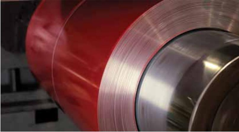
This picture shows the painted coil being rewound after slitting. Slitting is an off line process (separate from the coil coating process) in which a coil of material (master coil) is cut down into a number of narrower width coils. *Photo courtesy of Metal Coaters.*
