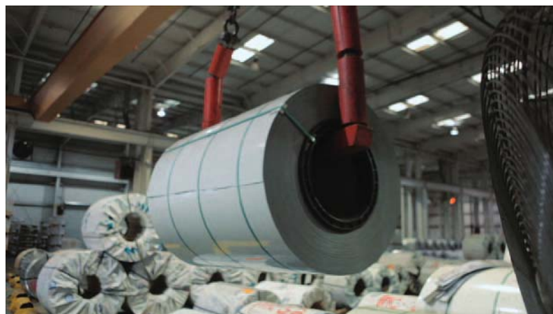
Metal coils from a supplier come into a metal coater for treatment eliminating more costly appliance manufacturer in-house processing. Source: Metal Coaters
