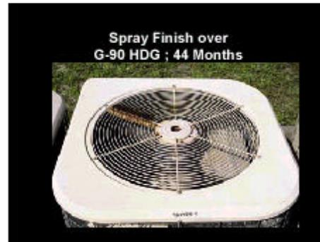
The enhanced corrosion resistance observed when using prepainted sheet as compared to other post painted methods of application is so significant, that in many cases metallic coating weights may be reduced. The photos below show the differences between a prepainted, G-60 hot-dipped galvanized part as compared to a spray, post painted, G-90 hot-dipped galvanized part after 44 months exposure at Daytona Beach:
